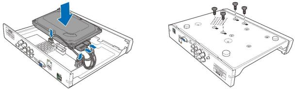
(3) Put the upper cover back carefully, and fix the cover with screws.
